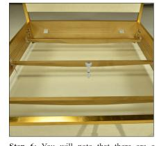
Step 6: You will note that there are a number of horizontal grooves running around inside of the frame at different heights. These allow you to mount the support slat and support brackets at different heights depending on the thickness of your mattress box. Decide which is most appropriate for your mattress box and secure the brackets and support slat as indicated in the diagram. Make sure that they are all at the same height to ensure maximum support for the mattress box.
