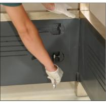
**Step 2**: Insert bolt with the half-moon spacer through the side rail and into the headboard. Tighten to secure. Repeat the procedure with the second bolt.
