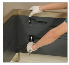
**Step 4**: Insert bolt with the half-moon spacer through the side rail and into the footboard. Tighten to secure. Repeat the procedure with the second bolt.
